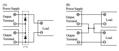
(\*1)Please select a bypass diode with maximum forward current rating more than output load current. And maximum reverse voltage must withstand each power supply output voltage.
